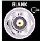
BLANK Output of blanking signal for the sweep operating mode.
